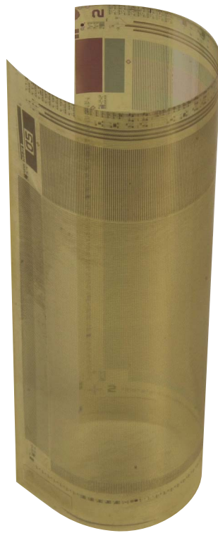
50 x 50 mm a-Si TFT array on 3 μm thick freestanding polyimide layer made by the EPLaR™ process. (Courtesy Philips Research)
