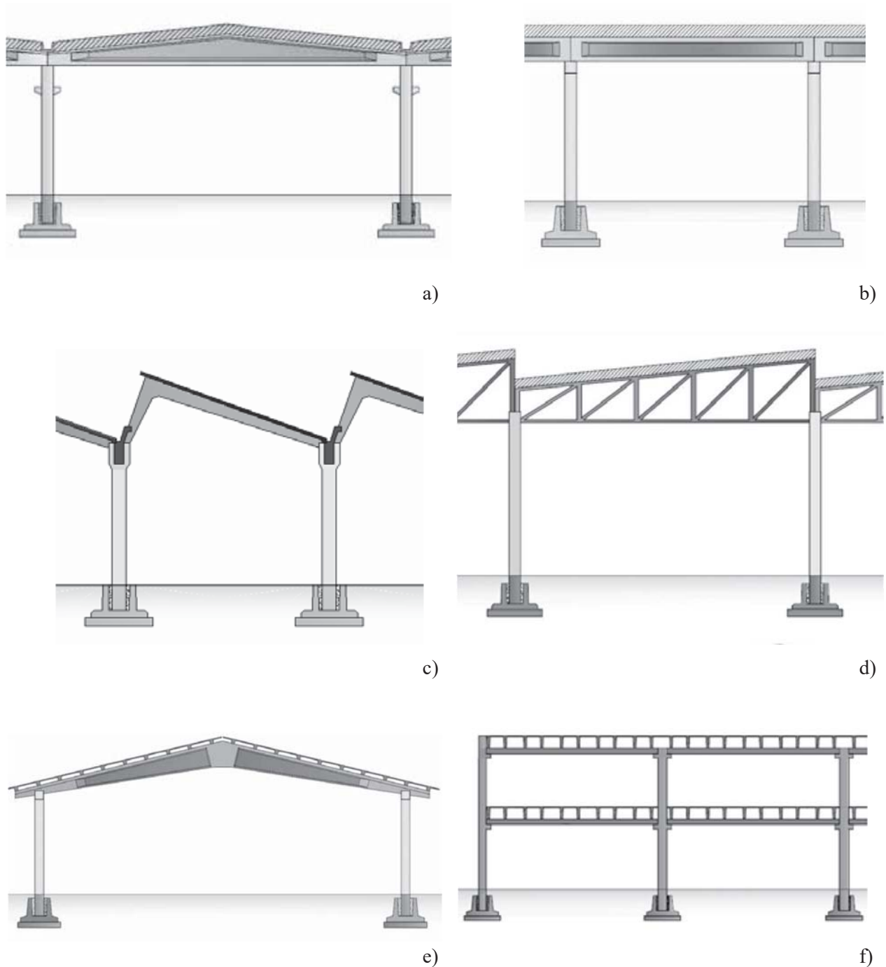
Figure 6-14 – Main typologies of precast structures in Italy (from Reluis 2008): a) Double slope beams; b) Planar roof structures; c) Shed structures; d) Truss structures; e) Boomerang beams; f) multistory structures with cantilever columns.
