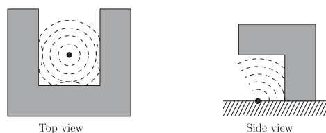
Figure 2-2 – Effect of the shape of the building on the shock wave and the pressure generated by it (da fib 2012).
