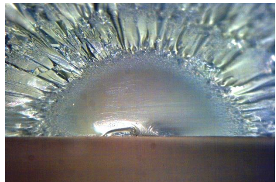
Figure 2.2. (a) Modification factor Y of a semi-elliptical crack, in the direction of its smallest axis ( \beta = 0^\circ ) and largest axis ( \beta = 90^\circ ), as a function of the ratio a/b between the dimensions of the crack in the two directions; (b) Fracture mirror of a plate broken by means of a four-point bending test.
