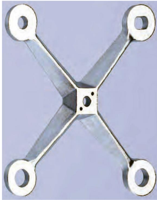
Figure 8.27. An example of an intermediate “spider” type support. Note the different holes at the four ends, which allow the connecting pins to move in specific directions.
