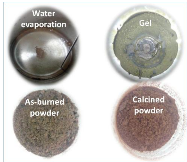
Fig 8: Flowchart with the solution combustion-based procedure used for the samples preparation and pictures showing selected steps of the synthesis
