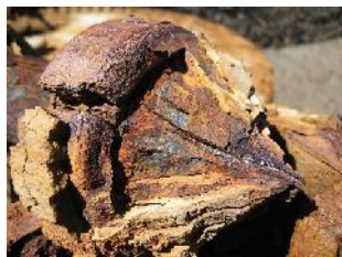
Fig. 1 Corroding iron machinery at the abandoned White Island Sulphur mine [4].
