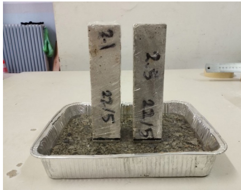
Figure 4. Specimens wrapped in PP plastic with the bottom part in contact with water.
