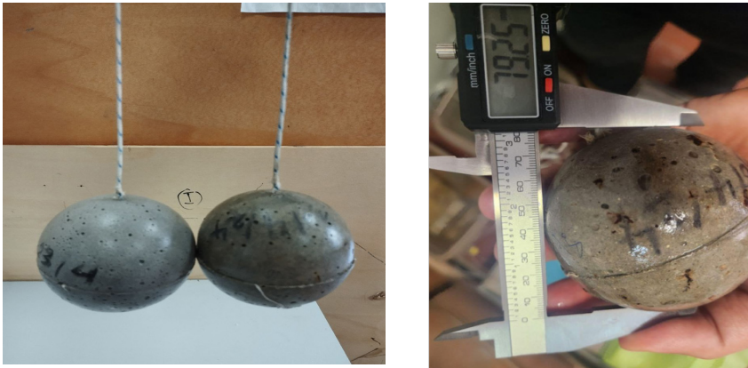
Figure 7. Details of the specimen geometry and position of the thermocouples employed inside the sphere.
