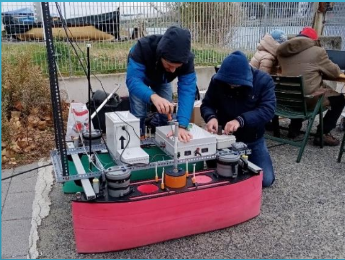
Installation of the spectroscopic sensor on a marine drone and drone in action in the area of Genova (Italy) port
