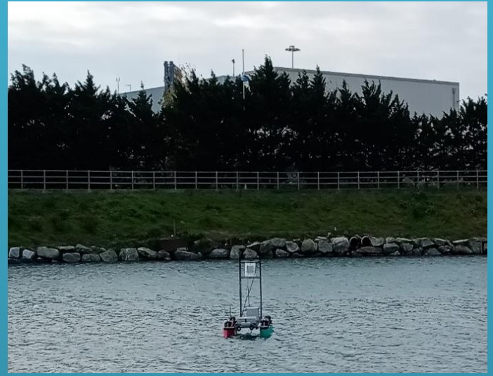
Installation of the spectroscopic sensor on a marine drone and drone in action in the area of Genova (Italy) port
