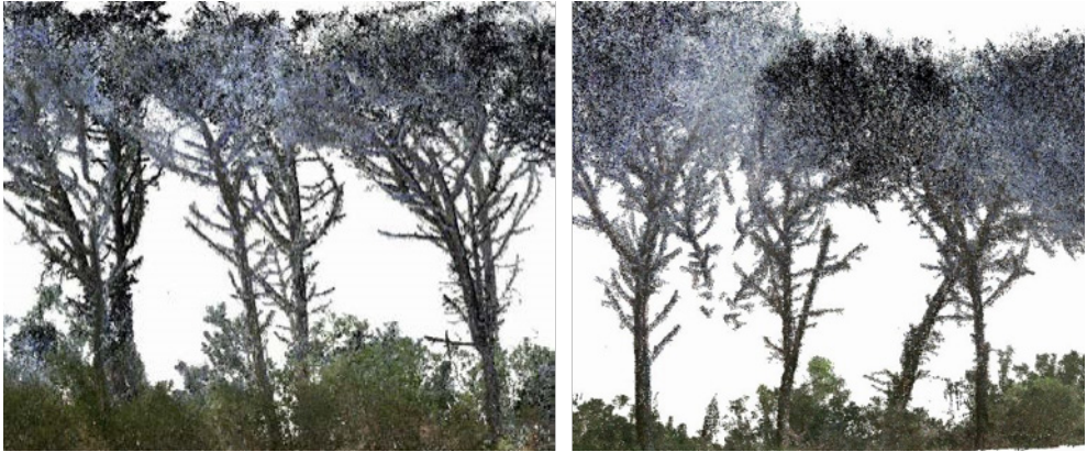
Example of point cloud generated by TLS scans in the coniferous stand with different degree of vertical fuel continuity.
